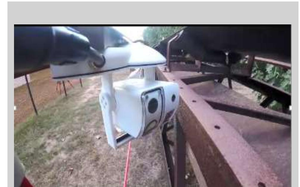
Robotic inspection vehicle on a rail. Automatic inspection on a regular schedule, and automatic upload and download of data to the ABB Ability™ cloud.
